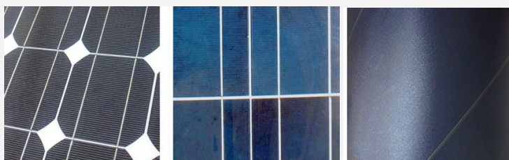
Figure 5: Different types of solar PV modules: monocrystalline silicon, polycrystalline silicon, thin-film Photos: Green Sun Rising
