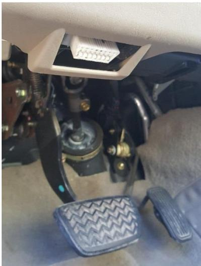
ii. Route the cable from the OBDII connector and plug the small end of the cable into the back or side of the Multifunction Vehicle Trip Computer.
